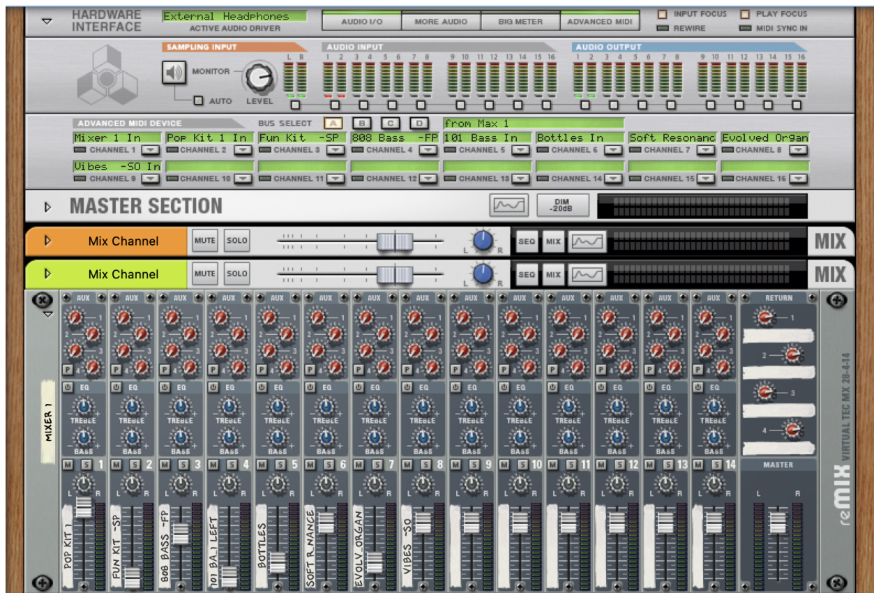
Figure 13: MMM Reason rack interface and mixer. Channel 1 on the interface is the mixer, while channels 2-9 are different instruments. Mixer channels 1-8 correspond to each instrument in the same order as the interface. Each instrument type comes in pairs of two, in the order: drums, bass, chords, lead.
